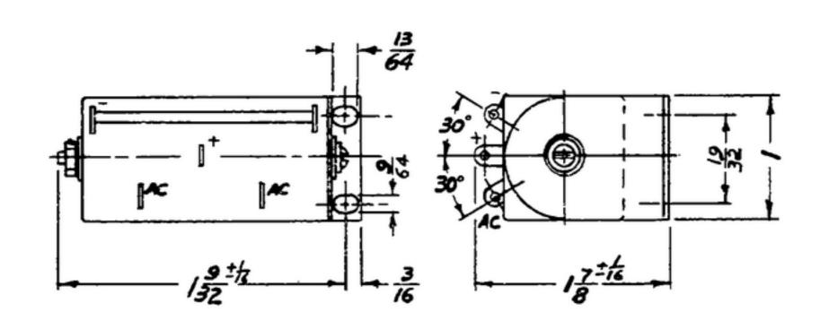
PART MAY BE TYPE EW 1023 AS SUPPLIED BY FANSTEEL METALLURGICAL CORP., CHICAGO, ILL., OR EQUAL, PROVIDING IT MEETS THE FOLLOWING REQUIREMENTS AND DIMENSIONS SHOWN.
